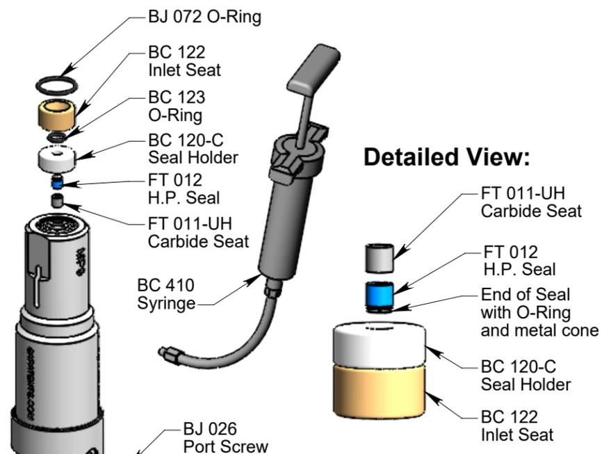
The Barracuda® uses ATF (automatic transmission fluid) for lubrication. It is recommended that a full syringe of fresh fluid be added to the swivel after every 20 to 40 hours of operation.
